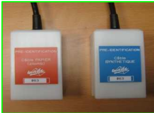
Sensors for «cable identification in short circuit»
