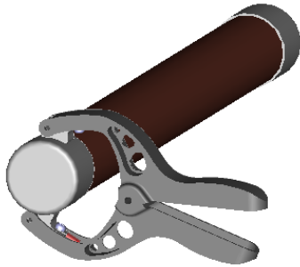
Placement of the clamp on the fuse
