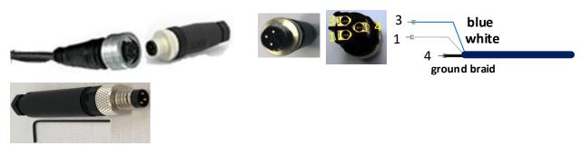
Warning: the earth cable must be as small as possible. Use the Allen key supplied for the wiring
