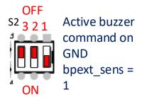
2 actions for configuration are to be performed: Position the switches on the CPU board Configure the option with the software
