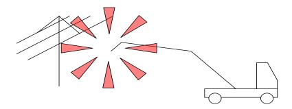
**DLDS** works on 11KV cables from 20 meters; the alarm distance is measured in free field (unobstructed).
