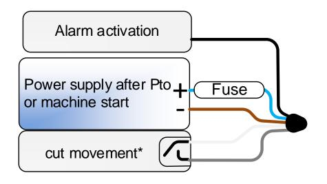
Alarm activation: factory configuration in + 12 / 24V
