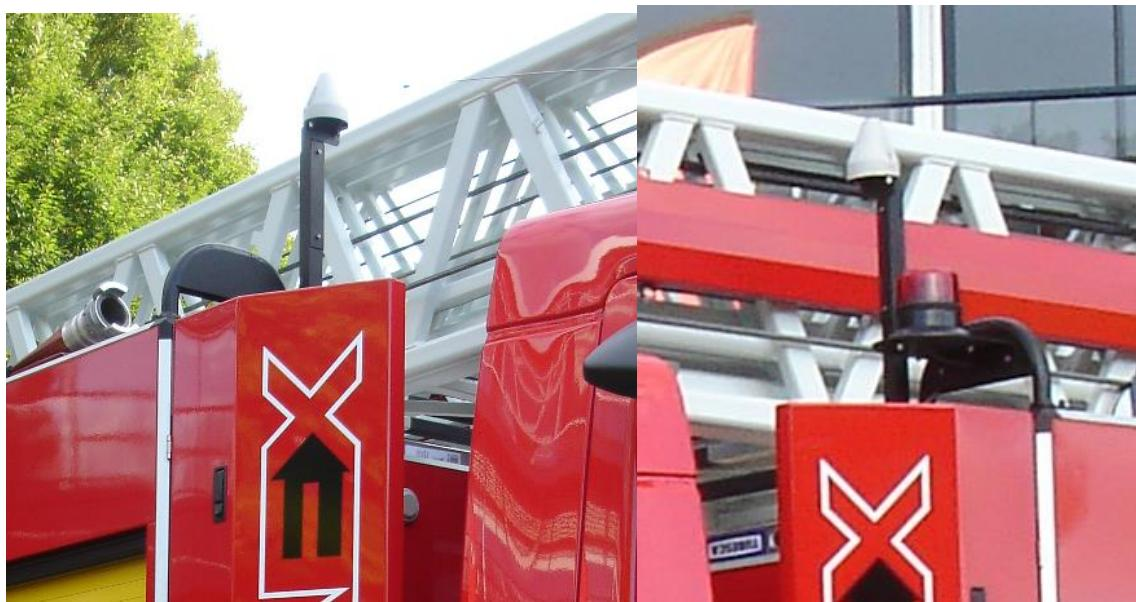
The ideal position is 20cm lower than the upper level of the large ladder.
