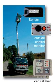
SKY NG NACELLE is a detector of high voltage lines : MV (< 50 kV) and HV (> 50 kV). SKY NG NACELLE warns the user with an acoustic and visual signal when the lifting device enters a danger zone at a distance between 3 and 6 m of a high voltage line.
