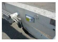
Put the battery cover back to its place and the sensor back to its magnetic base. Verify that the base is well fixed as well as the link cable.
