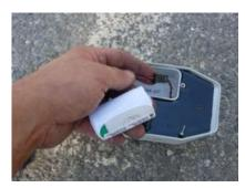
Unscrew the battery cover and unplug the connector.
