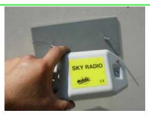
With a wrench of 7mm remove the sensor from its magnetic base.
