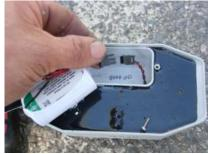
Replace the lithium battery including its connector for sensor Ref. : SKR\_CAP\_110SKR\_PIL\_110.
