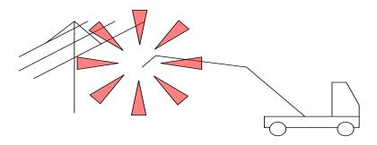
SKY NG RADIO 2 works on 15KV cables from 6 meters; the alarm distance is measured in free field (unobstructed). SKY NG RADIO 2 does not work on power lines less than 15 kV.
