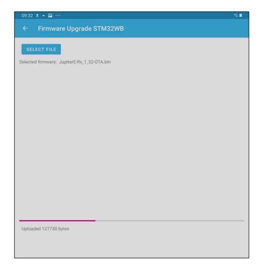
Wait for the update to complete, and check that the version displayed on the device (transmitter or receiver) start-up screen is the correct one.
